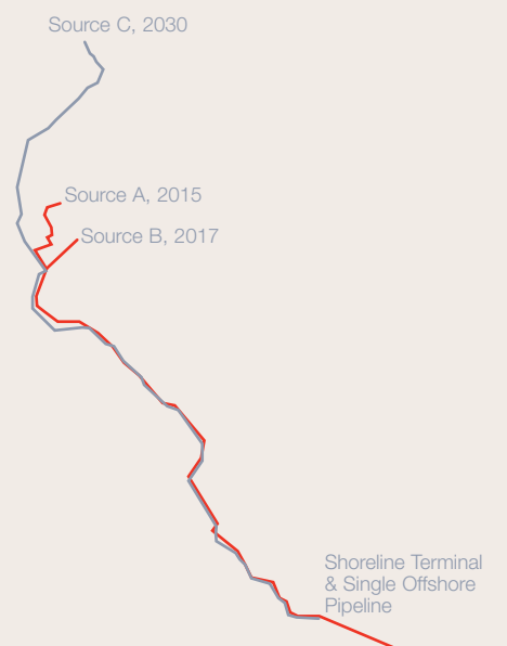
Figure 6.1 Example of phased network pipelines
